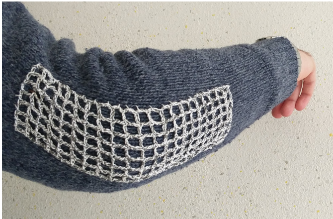
Fig. 2: The piezo-resistive sensor integrated in the sweater.
